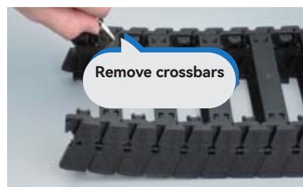
Insert screwdriver into the slot. Using a lever action, release the crossbars
